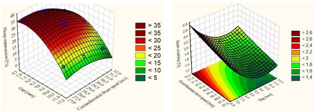
**Fig. 3 – Responses surfaces of heap separation and grain crushing to alternative drum operating speed and gap between the deck's ribs dependencies**
